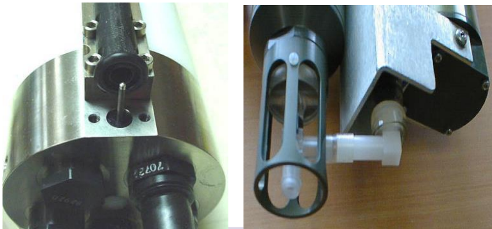
SBE 9plus CTD in cage (shown with standard T & C sensors & pump)
