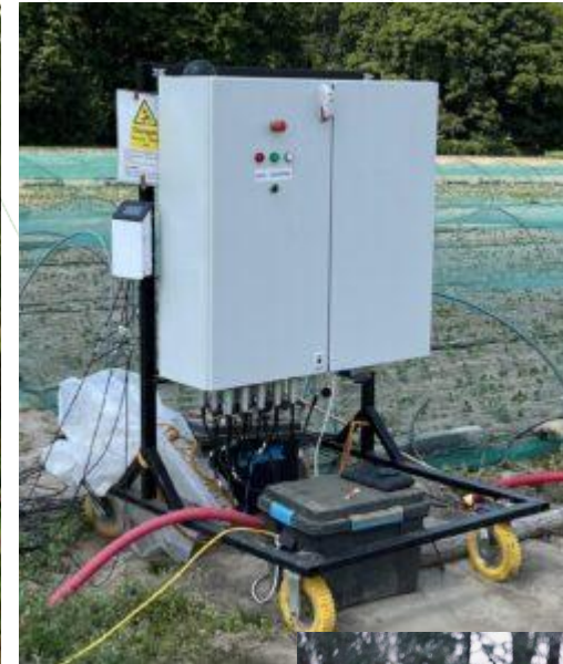
ERT Monitoring system from Subsurface Insights
