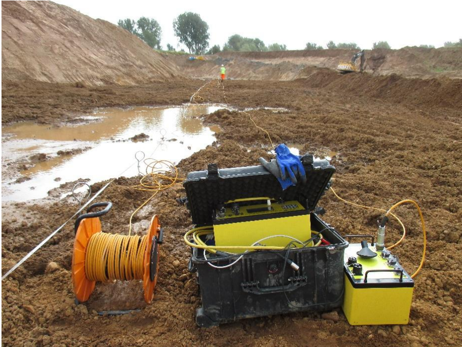
AGI SuperSTING R8/IP & Switchbox
