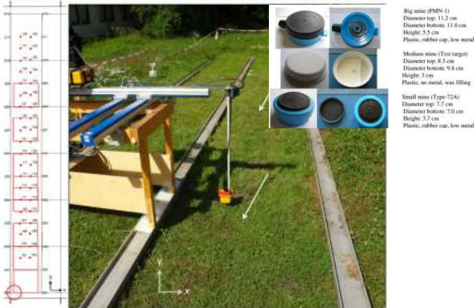
measurement layout: red squares denote the surveyed areas, red points indicate targets' positions
