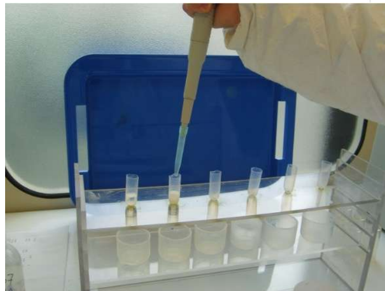
Boron procedure: Specific ion-exchange resin (Amberlite) TONARINI ET AL 1997
