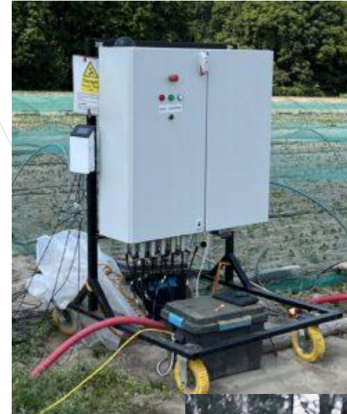
ERT Monitoring system from Subsurface Insights
